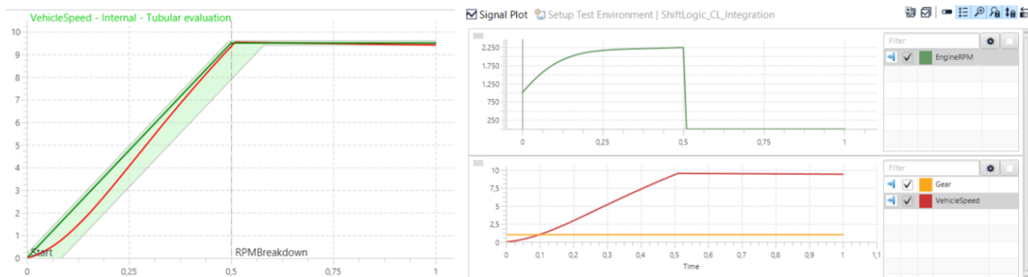
Evaluation view of VehicleSpeed (left; with reference signal and tolerance tube shown) and recorded values for EngineRPM , Gear , and VehicleSpeed (right)
